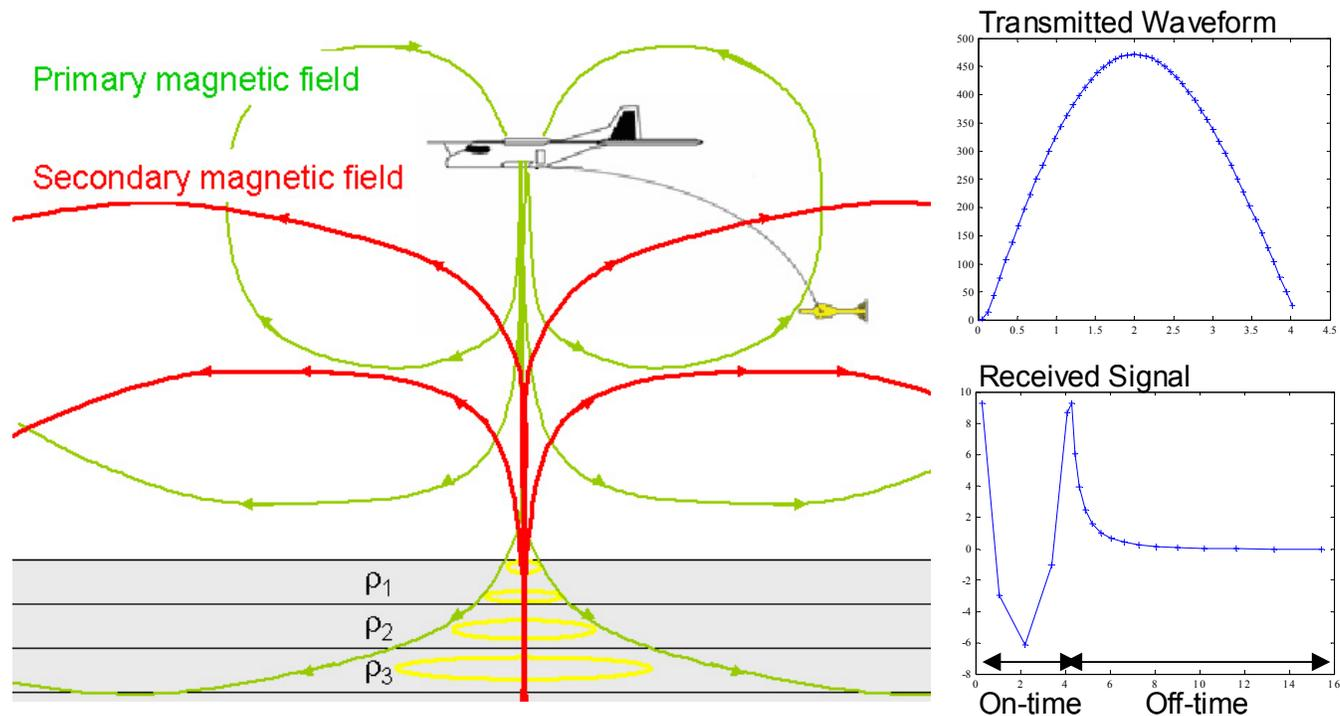
Figure 1. Basic principles of airborne TDEM surveying. Voltage versus time plots illustrate the transmitted waveform and a typical received signal. The present study seeks to invert the data recorded during the transmitter off-time for subsurface resistivity structure.
