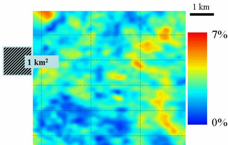
**Figure 3.** Fast velocity – slow velocity time slice, Rocky Mountains showing channel with high anisotropy embedded in shales and mudstones with low anisotropy.
