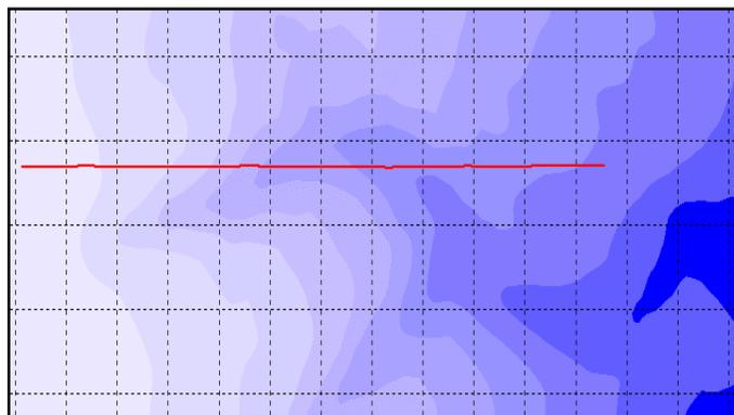
**Figure 1:** Water depth map. Depths range from 600 m (pale blue) to 1400 m (dark blue). The grid lines spacing is 1km. The shot locations follow the red line from right to left.
