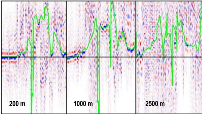
**Figure 3:** Cross-correlations between the input data and the 2D predicted multiples for 3 offset planes (as indicated), for a short window around the first-arrival multiple. The maximum lag is 100 ms. The green line indicates the predicted error from the error analysis.
