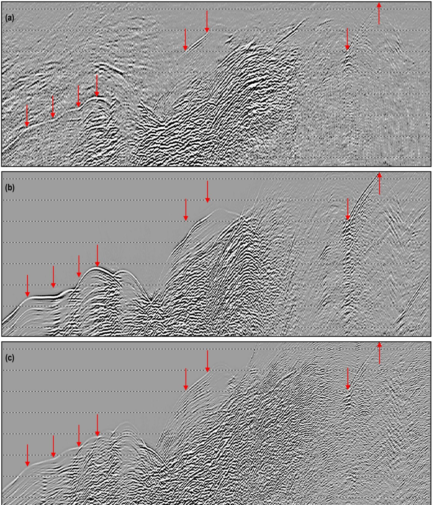
**Figure 2:** The 200 m offset plane at the level of the first-arrival multiple (arrowed) for (a) the input data, (b) 2D predicted multiples, and (c) 3D predicted multiples. Note that these plots are reversed with respect to figure 1, i.e. the sailing direction was from left to right.
