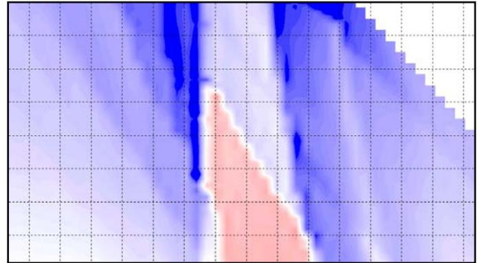
**Figure 4:** Crossline aperture as a function of shot location (horizontal axis) and offset (vertical axis). Deep red and deep blue correspond to  $-700$  m and  $+700$  m respectively.
