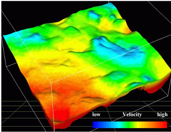
Figure 1. Velocity distribution in the reservoir layer obtained by tomographic inversion. Velocities vary linearly with depth as  $V(z) = V_0 + k z$ , with a constant gradient  $k$  and laterally variable  $V_0$ .
