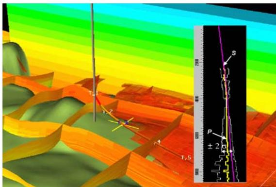
**Figure 4.** 3-D display of predicted  $P$  within the reservoir with slice through calculated overburden pressure cube. Well planning with automatic extraction of pore pressure predictions and associated confidence margins may be used to calculate a safe mud weight window by stochastic simulation.
