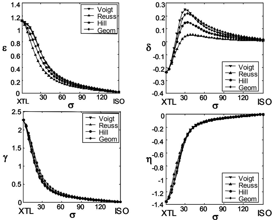
Fig. 3. Anisotropic parameters for TI medium as a function of texture. Right end of the ordinate axis for each plot represents values of fully aligned polycrystalline with the properties of a single crystal (XTL). All parameters approach zero for an isotropic aggregate. Notice dependence of  $\varepsilon$  and, especially,  $\delta$  on the averaging procedure. Anellipticity ( $\eta$ ) values are very close for all approximations.
