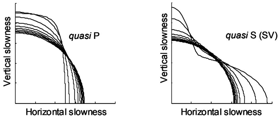
Fig. 4. Slowness surfaces for  $qP$  and  $qS$  (SV) waves for intrinsically anisotropic shale of TI symmetry calculated from the elastic constants obtained by the GMA procedure. Slowness surfaces vary from highly anisotropic for a single crystal to almost circular for *quasi* isotropic aggregate.
