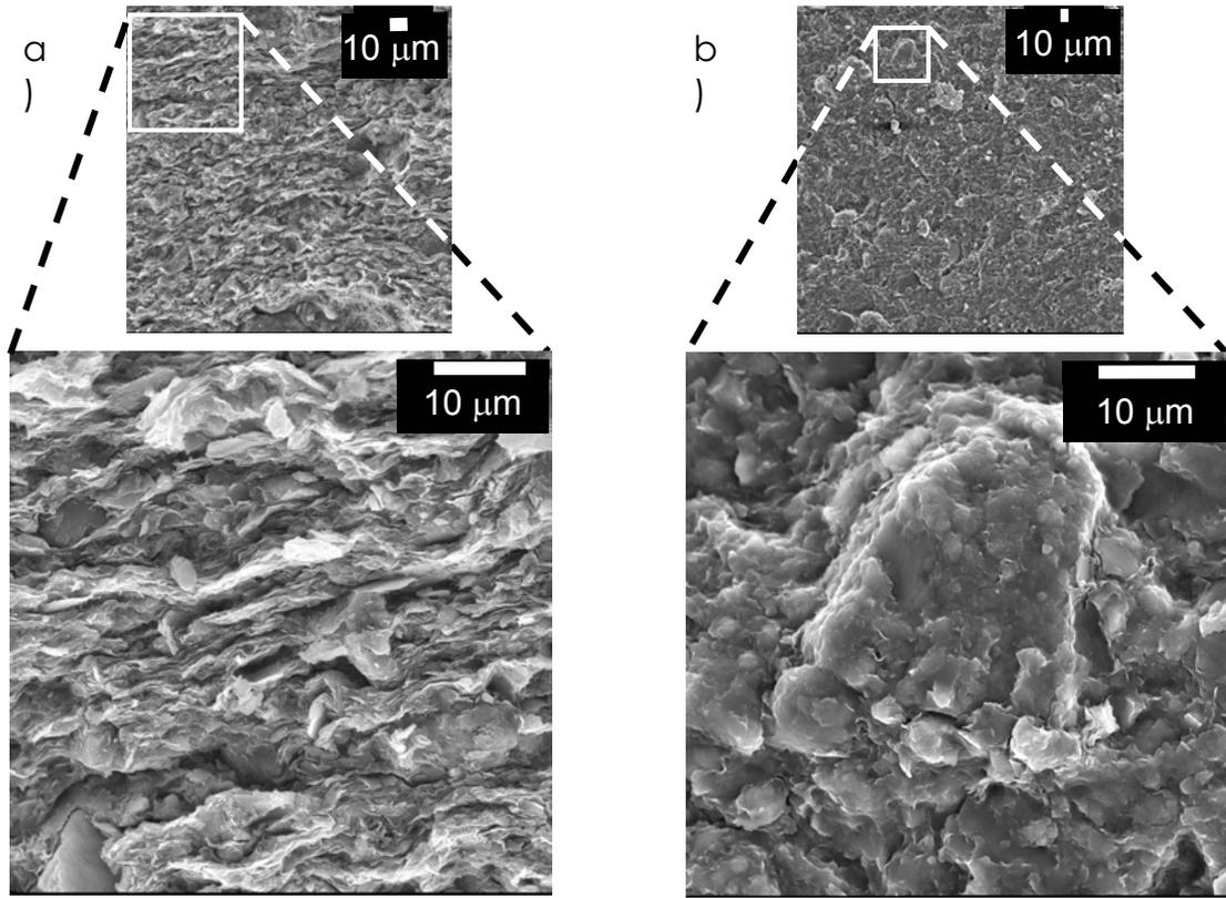
Fig. 1. SEM image SEM images of Colorado Shale from the Cold Lake area of Alberta, Canada: a) section perpendicular to the bedding plane; b) section parallel to the bedding plane. Average size of clay platelets is several microns and almost order of magnitude smaller than embedded randomly distributed silt (quartz, calcite etc.) particles.
