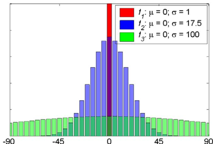
Fig. 2. Schematic representation of shale texture by Gaussian distributions with different standard distributions (not to scale).
