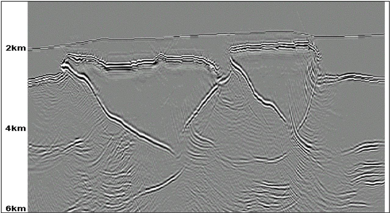
Figure 4. Wave equation shot record PreSDM of the synthetic data with model derived from the data (tomography plus CIG analysis). The image of the turbidites is strongly distorted.
