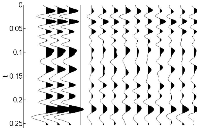
Figure 1. A pilot trace (repeated three times for visibility) and a trimmed stack. Each of the 10 stacked traces consists of a stack of 50 random noise data traces that have been cross-correlated against the displayed pilot trace.
