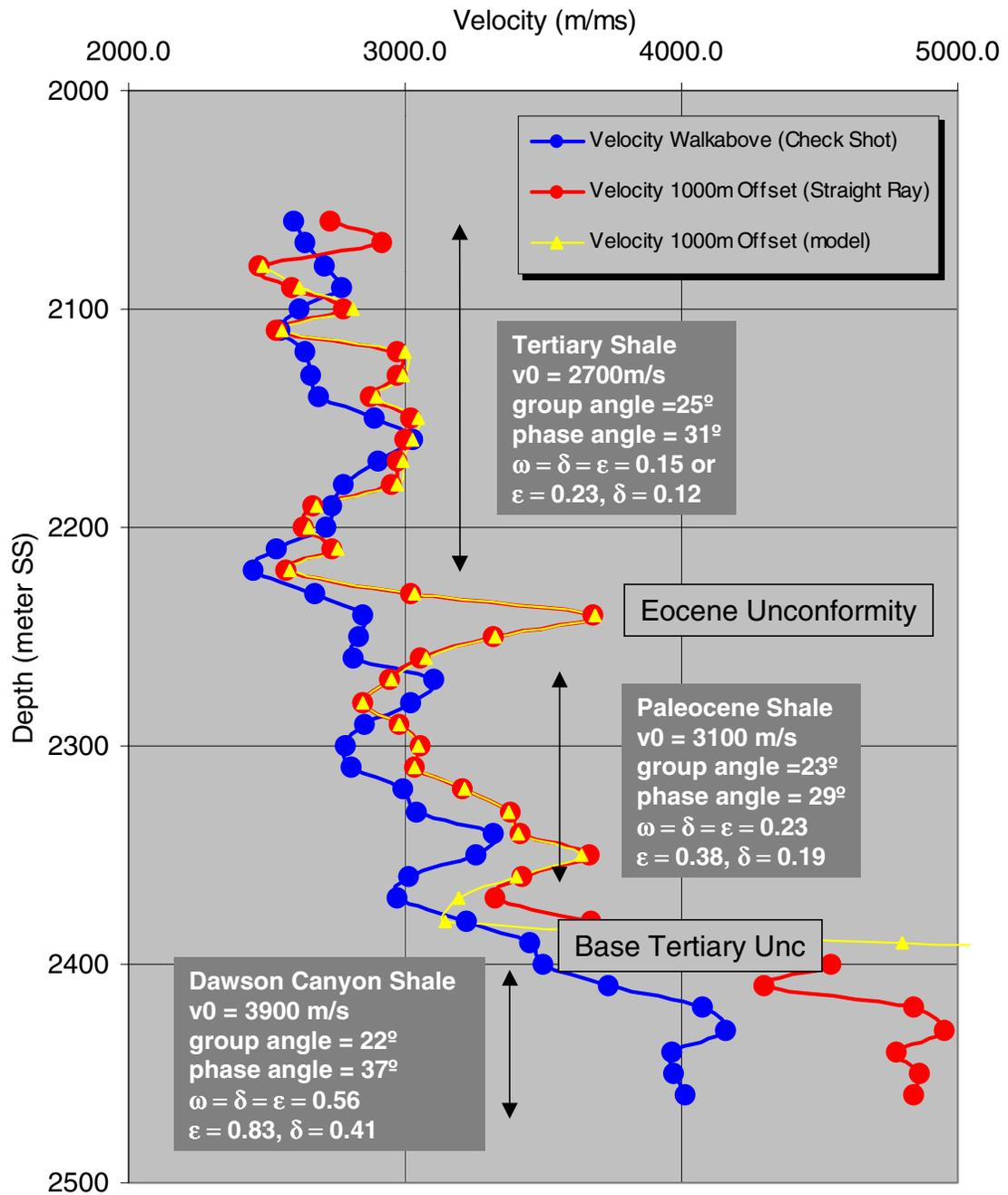
Figure 2: White Rose H-20 Interval Velocity Profile - The blue line represents the velocities for the zero offset VSP, the red line for the 1000-m offset VSP using a straight line geometry and yellow using the raypath length from the GXII model.
