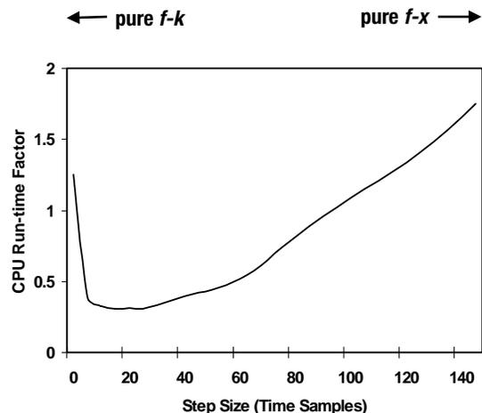
Figure 6: Measured cost tradeoff curve for hybrid datuming.
