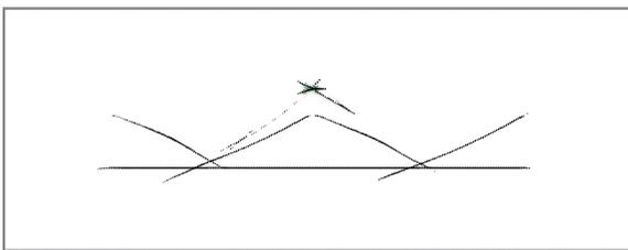
Figure 5: Migration with an incorrect, low velocity after static time-shift datuming
