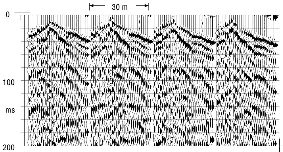
Figure 2. Presumed 'inline' horizontal component receiver gathers from the 2000 Belize high resolution 3-C seismic survey.
