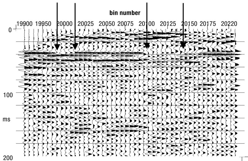
Figure 4. CCP stack of 'inline' component after wavefront healing, Kirchhoff migration and predictive deconvolution. Remarkably high frequencies are recovered for the events between 40 and 60 ms.
