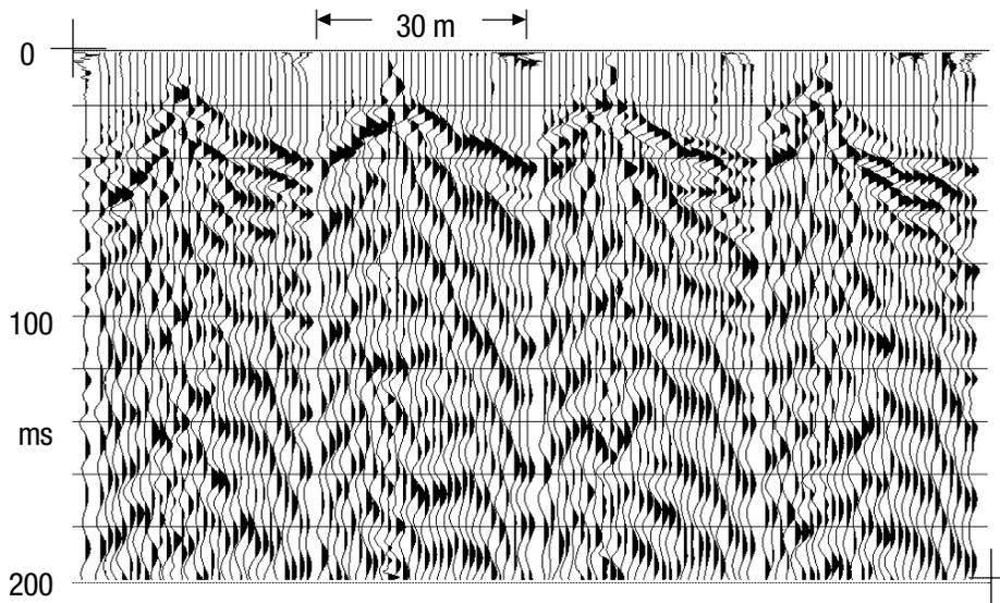
Figure 1. Presumed 'vertical' component receiver gathers from the 2000 Belize high resolution 3-C seismic survey.
