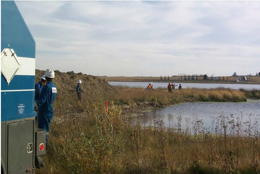
Figure 1. Deployment of the wireline across the "lake". The 5-level, 3-C VSP tool was attached at the far side of the lake and winched back to provide different receiver positions for the onshore vibrator.
