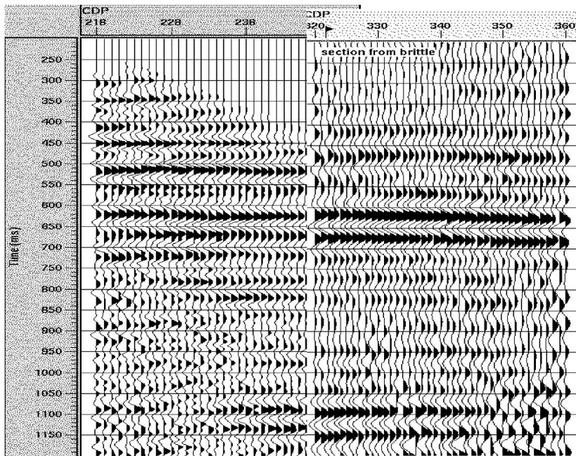
Figure 4. The stacked section for vertical component of slough data was shown on the left. The comparison of stacked section of lake-bottom cable with surface seismic section was shown on the right.
